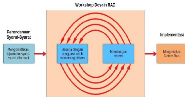
Gambar 3.1. Tahapan Rapid Application Development
